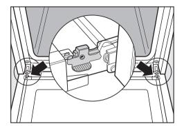
The oven door is connected to the oven by hinges.
